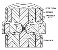
Fig. 2 "Closed" View of the Belt High Pressure, High Temperature Apparatus
